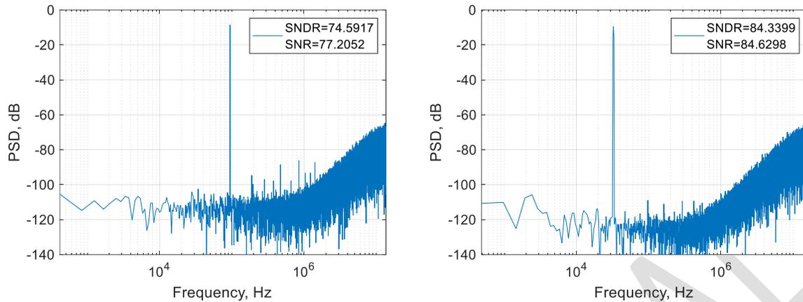
Figure 6: Panther 3: 2<sup>nd</sup> order noise shaping with a 6-bit core SAR and two independent 1<sup>st</sup> order feedback loops, (a) Silicon results and (b) simulation results.
