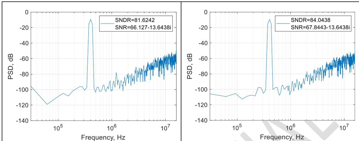
Figure 4: Simulated results of Analog core extracted (without calibration left and calibrated right)
