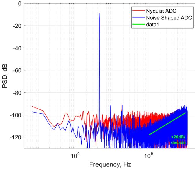
Figure 5: Panther 2v3 measurements on a Fibbed chip showing SNR with and without noise shaping. SNR improves from 69.8dB to 75dB when NS is turned on
